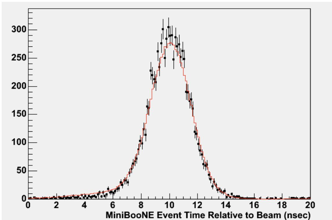
Figure 4: A comparison between the absolute timing of MiniBooNE muon-neutrino charged-current quasielastic (CCQE) data events relative to the beam (black histogram) and the Monte Carlo expectation (red curve).
