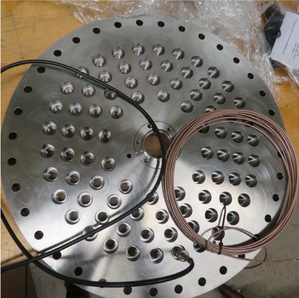
Figure 3: A photograph of one of the two 80 channel feed-through plates.
