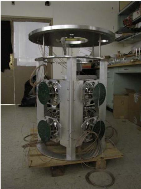
*Figure 1: A photograph of the inside of the cryostat that is testing eight PMTs at a time in liquid argon.*
