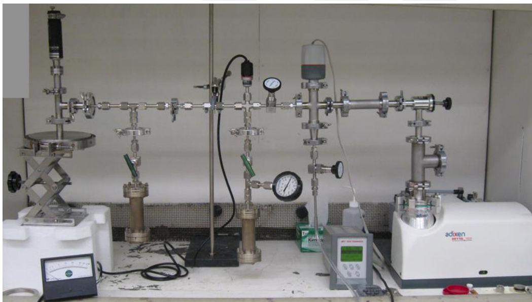
Apparatus to be employed for the extraction of ^{39}\text{Ar} gas from an irradiated KCl target.
