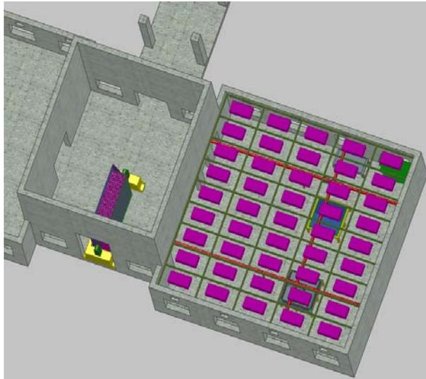
*Figure 3: A schematic drawing of the ECAL factory layout. A larger door will be required to get a 4m x 4m downstream ECAL out of the building.*
