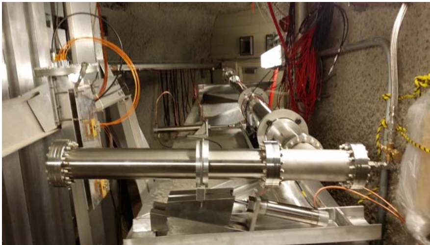
Figure 1: A photograph of the Cherenkov detector in the NuMI alcove.
