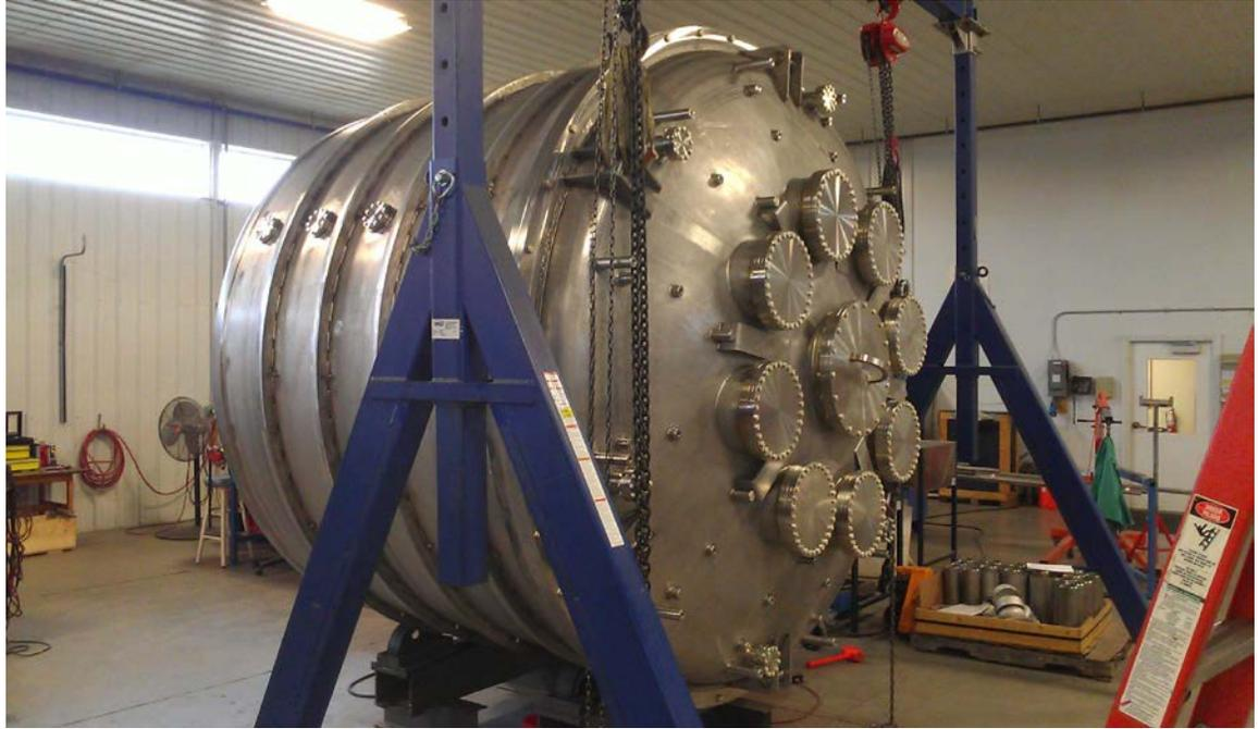
**Figure 2:** Photo from March, 2014, of the CAPTAIN cryostat on the floor at the vendor. The inner vessel passed the pneumatic pressure test. Helium mass spectrometer leak tests are on-going.
