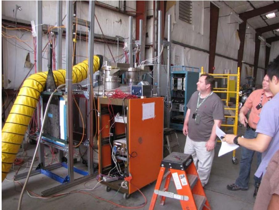
**Figure 2: the CAPTAIN prototype detector is filled with liquid nitrogen.**
