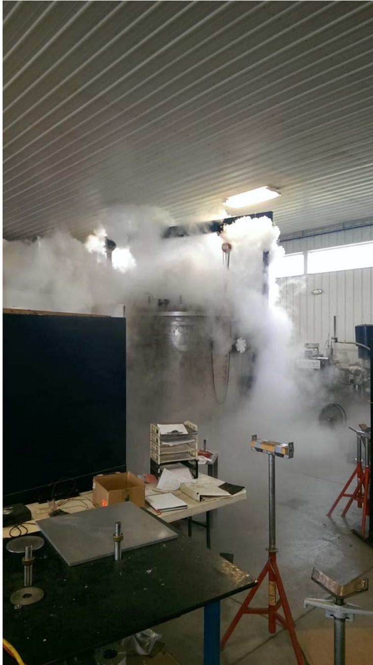
**Figure 3: Photo from June, 2014, of the CAPTAIN cryostat on the floor at the vendor being cold shocked with nitrogen.**
