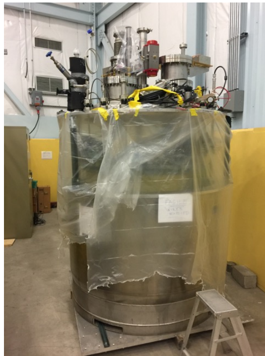
Figure 1: MiniCAPTAIN cryostat open for electronics testing after moving to LANSCE WNR in March 2017.
