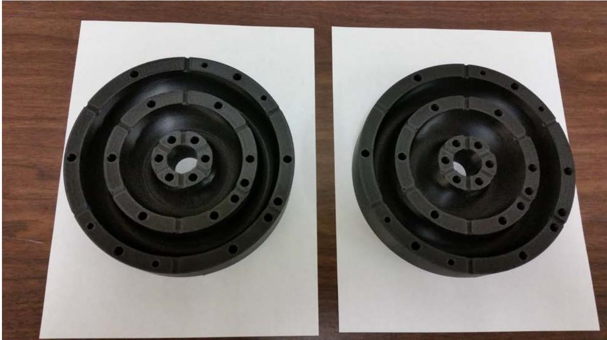
Figure 2: Printed cavity halves.
