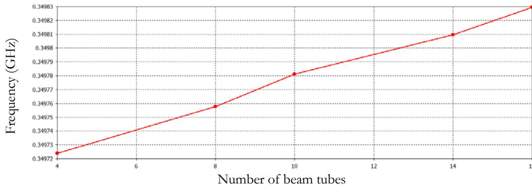
Figure 1: cavity frequency dependence with number of beam tubes.
