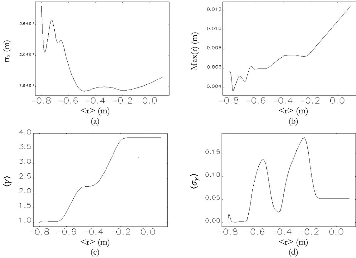
Figure 2: (a) rms and (b) envelope of the beam as a function of radius, and (c) mean and (d) RMS variation of the Lorentz parameter as a function of radius.
