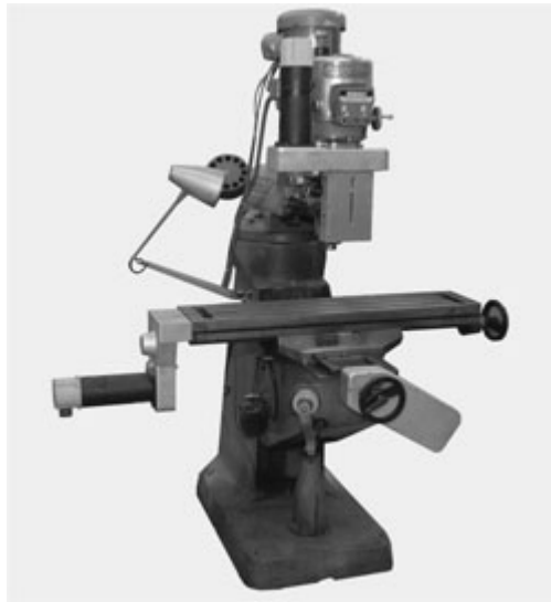
Figure 1.9: Bridgeport mill with CNC retrofit [32]
