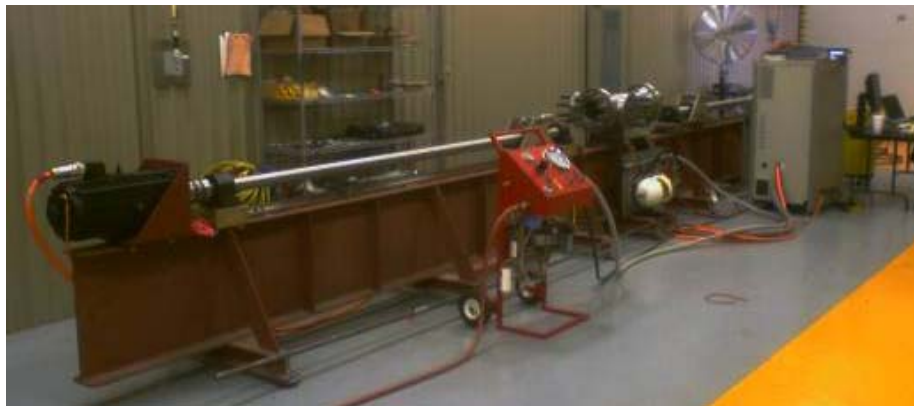
Figure 5.1: Scaled seal testing system [45]
