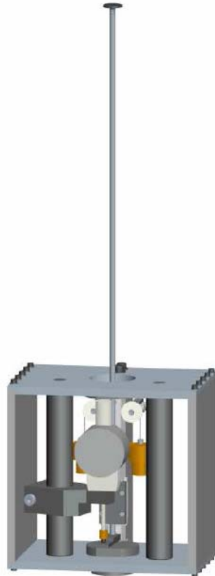
Figure 5.6: Strain gauge module [65]
