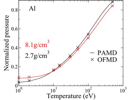
FIG. 3. (Color online) Comparison of pressure for an aluminum plasma between PAMD and OFMD in the Thomas-Fermi approximation. We show total pressure divided by the pressure of a fully ionized aluminum plasma of non-interacting classical ions and quantum electrons. Excellent agreement is found for both densities across this wide temperature range.
