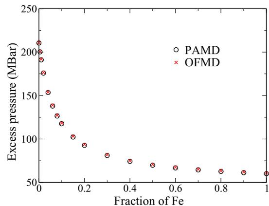
FIG. 4. (Color online) Excess pressure for a mixture of iron and helium at  $10\text{g/cm}^3$  and  $50\text{ eV}$  from PAMD and OFMD [26] in the Thomas-Fermi approximation. Excess pressure is defined as the total pressure minus the ideal ion contribution (see Ref. [26]). We find excellent agreement for all mixing ratios.
