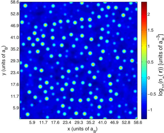
FIG. 2. (Color online) Two-dimensional (2D) slice of electron density in the Kohn-Sham version of the model for aluminum at  $8.1\text{g/cm}^3$  and  $1\text{ eV}$ . The plot shows  $\log_{10}$  of the electron density. For reference  $\log_{10}$  of the average total electron density is  $-0.46$  and  $\log_{10}$  of average screening (valence) electron density is  $-0.99$ . The ion positions were generated in a molecular dynamics simulation with 5000 nuclei using periodic boundary conditions.
