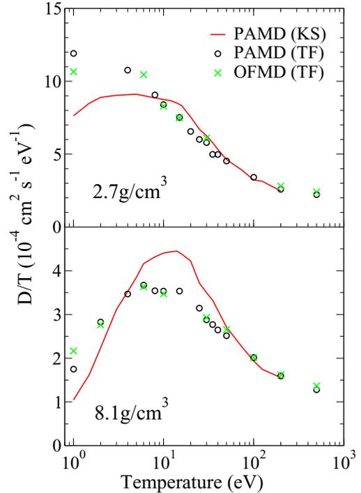
FIG. 5. (Color online) Comparison of the self-diffusion coefficient  $D$  for aluminum between PAMD and OFMD in the Thomas-Fermi approximation. Also shown is the PAMD calculation using the Kohn-Sham functional from 1–200 eV. Such a calculation would be a formidable task for the *ab initio* KS-DFT-MD method. Note that we plot  $D$  divided by temperature in eV.
