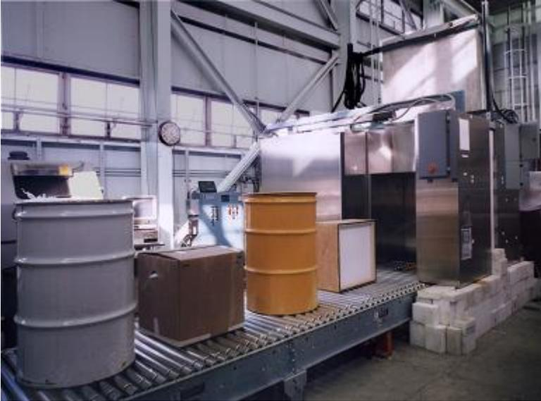
*Fig. 6. The output side of the shuffler has a longer conveyer section to allow containers to be stored while new containers are assayed. Shown here are 200-liter drums, a HEPA filter, and a cardboard box*
