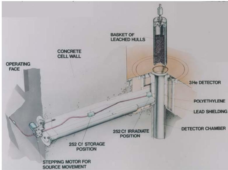
Fig. 8. The components of the Dounreay shuffler. A cylinder of polyethylene extends through the hot cell wall and the  $^{252}\text{Cf}$  source is stored in the center of the wall. A basket of waste is lowered into the assay chamber while measurements are taken. The electromechanical components are in the corridor on the left edge of this drawing.
