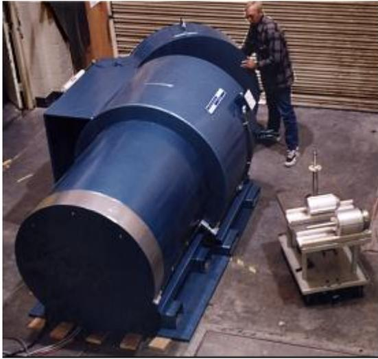
*Fig. 3. Ed Adams opens the door to the assay chamber of the Billet Shuffler. The large cylinder in the foreground stores the  $^{252}\text{Cf}$  source. Two simulated billets are on the cart to the right.*
