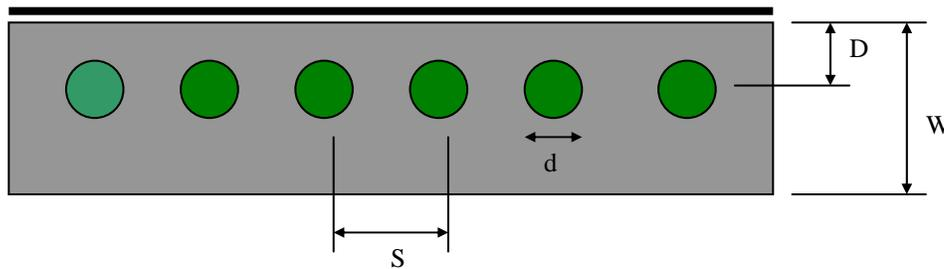
*Fig. 18. A detector bank consists of  $^3\text{He}$  tubes embedded in polyethylene. The heavy line at the top is an optional layer of cadmium and stainless steel lining the assay chamber. The assay chamber is located above the cadmium and steel liner. The important geometric parameters are indicated.*
