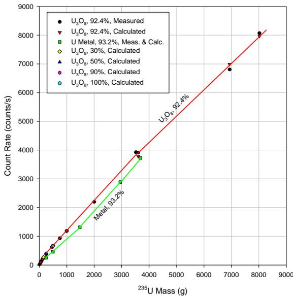
Fig. 14. The curve in red is the measured calibration for dry  $U_3O_8$ , 92.4% enriched. The effect of deviations from this have been calculated and are shown for comparison. Using metal disks (6-cm diameter) greatly reduces the count rate for the same mass of  $^{235}U$  because of self-shielding from the higher density (19 instead of 4  $g/cm^3$ ). Enrichment effects are better seen in Fig. 15
