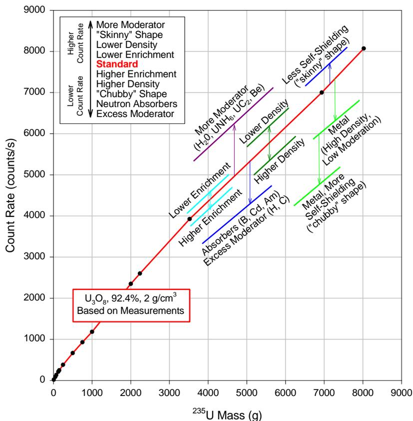
Fig. 13. When the material being measured has characteristics different from the calibration standards, the accuracy can be adversely affected. In this example, the calibration shown by the red line is for U<sub>3</sub>O<sub>8</sub> with 92.4% <sup>235</sup>U and 4 g/cm<sup>3</sup>. Potential changes are shown and the qualitative effect of each is indicated (exaggerated for clarity).
