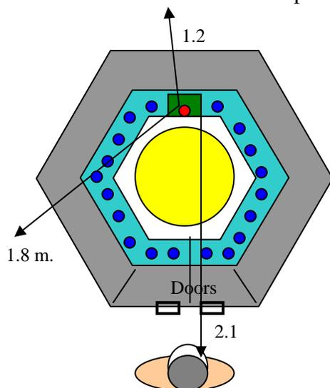
*Fig. 17. A horizontal cross section of the standard shuffler for 200-liter drums is shown with an operator positioned in front of the doors. A drum is surrounded by detector tubes embedded in polyethylene, which is wrapped with an outer layer of borated polyethylene and 1.2 cm. of lead to form the shielding. Distances to the  $^{252}\text{Cf}$  source and the amounts of shielding in the different directions are shown.*
