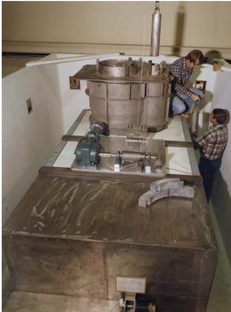
*Fig. 7. George Eccleston and Tom Van Lyssel assemble the Spent Naval Fuel Shuffler for testing. A container is suspended above a small tube where assays are done on waste material inside the container. A larger tube to the left is for the fuel assemblies. A motor in the center ran an automated hoist. The motor at the bottom of the photograph is the stepping motor for the  $^{252}\text{Cf}$  source.*
