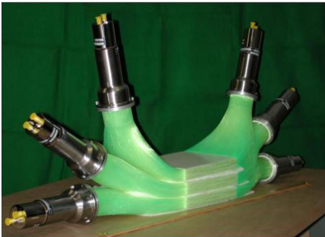
Fig. 14. Three of 12 NCCR detector elements are assembled to form one side of the four-sided neutron well counter. PMTs are coupled optically at the ends of each element. Signals from opposite ends of each element are combined into a single preamplifier. Note meter stick in foreground.
