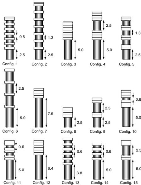
Figure 7.6. The 15 different configurations of uranium disks. The disks are represented by rectangles, and the aluminum spacers are shown as cylinders, with their heights given in cm. Each uranium disk has a mass of approximately 528 grams except for one which has about half the mass. The configurations labeled 3, 7, and 12 were used for calibration.
