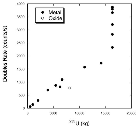
Fig. 7.4. Y-12 data on HEU metal and oxide samples measured in an AWCC. The observed doubles are plotted as a function of  $^{235}\text{U}$  mass (Ref.2).
