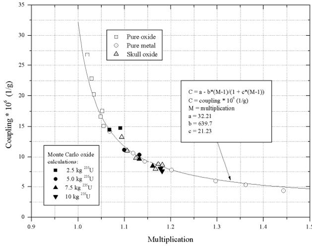
Fig. 7.1 Coupling as a function of multiplication for three categories of uranium samples (Ref. 6).
