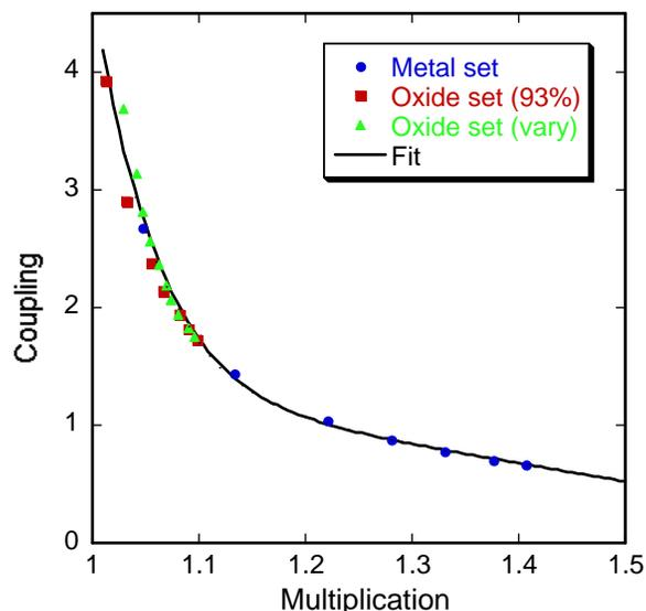
Fig. 7.2. The Monte Carlo modeled relationship between the multiplication and the coupling for three material types: uranium metal, uranium oxide of constant enrichment, and uranium oxide of variable enrichment. The black line is an empirical fit to all the data points (Ref. 10).
