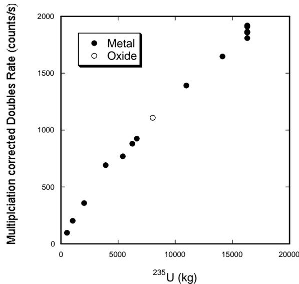
Fig. 7.5. Y-12 data on HEU metal and oxide samples measured in an AWCC. The triples-to-doubles ratio is used to correct the doubles response, and the self-multiplication-corrected doubles are plotted as a function of  $^{235}\text{U}$  mass (Ref.2).
