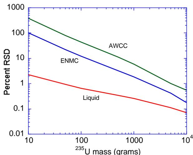
Fig. 7-3. Estimated RSD for the active multiplicity assay as a function of  $^{235}\text{U}$  mass (g) in uranium metal for the three detector options summarized in Table 7.1 with 1000-s counting times (Ref. 19).
