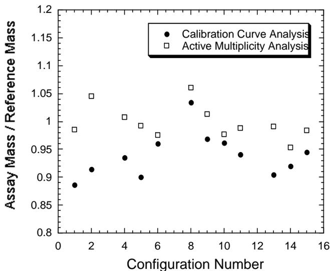
Figure 7.7. Comparison between the calibration curve analysis results (solid circles) and the active multiplicity analysis results (open squares) for the different HEU metal disk configurations. An unbiased result will have an Assay Mass / Reference Mass value of unity (Ref. 9).
