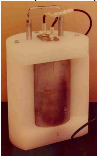
*Fig. 15. Shielded Neutron Assay Probe (SNAP-II) used for U and Pu holdup measurements in heavily shielded situations.*
