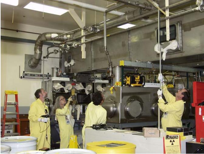
*Fig. 12. A compact NaI detector is shown during measurements of plutonium deposits in overhead ducts.*
