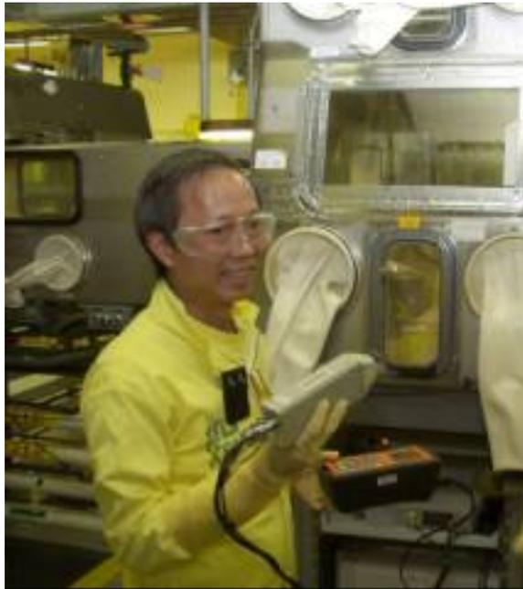
*Fig. 3. The Peltier-cooled CdTe detector is shown measuring Pu isotopics in a glove box.*
