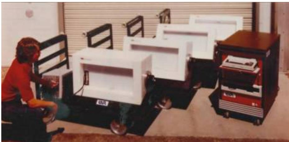
*Fig. 17. Wide-area neutron detectors used to measure holdup at uranium enrichment plants.*
