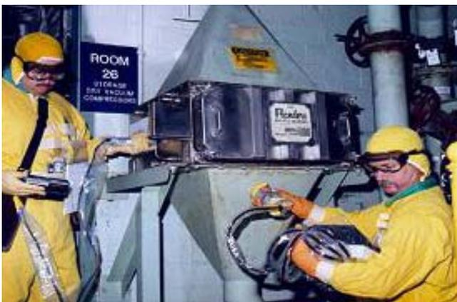
*Fig. 14. Measurements of  $^{235}\text{U}$  deposits in a filter system performed with CZT and NaI.*
