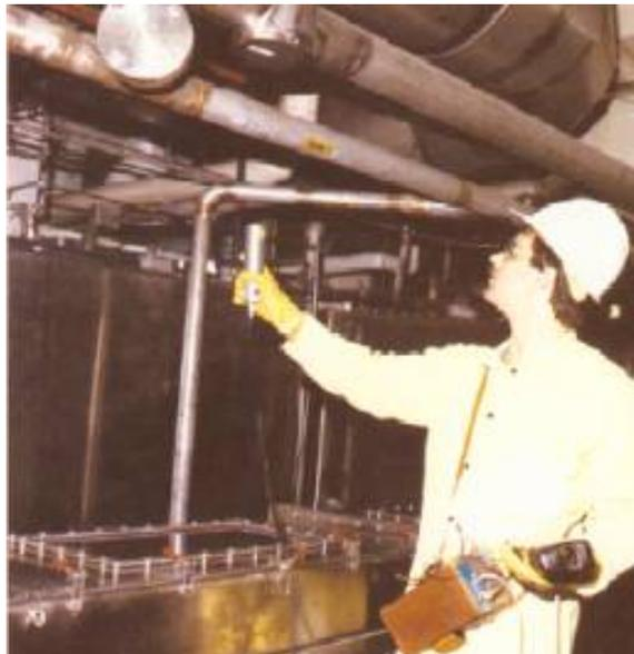
*Fig.11. GGH applied in a uranium facility to measure an overhead duct.*
