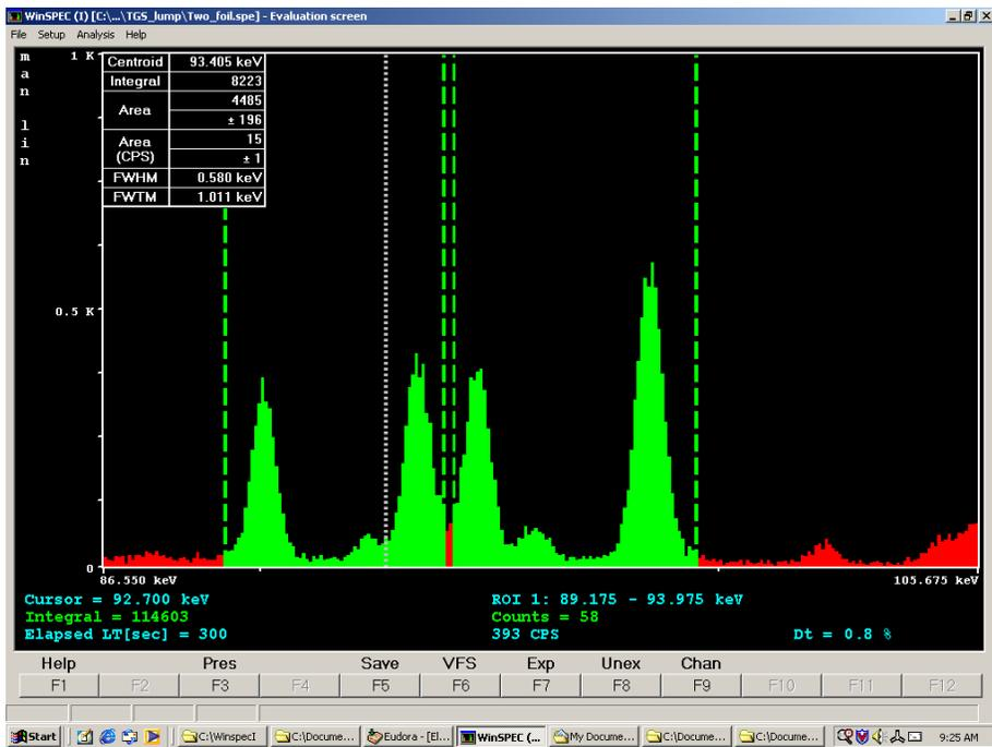
*Fig. 13 Comparison of the fluoresced uranium K x-rays with thorium K x-rays (from U decay) in a thick metal disk (upper spectrum) with those from very thin foils (lower spectrum). The lower energy ROI covers the Th K $\alpha$  x-rays and the higher energy ROI covers the U K $\alpha$  x-rays. Note the much higher relative intensity of the uranium x-rays from the metal disk.*
