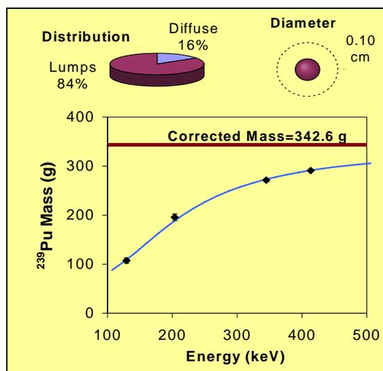
*Fig. 12 Lump Correction estimate of the mass of plutonium metal in a sample.*
