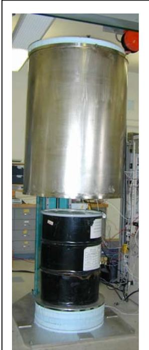
**Figure 13. Photograph of the LVC with the calorimeter in up position after the 208-l drum has been loaded. The circular insulation below the drum is the LVC pedestal.**
