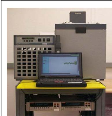
**Figure 12. Picture of a high-precision solid-state calorimeter in a water bath. The IBM laptop in the foreground is used for data acquisition.**
