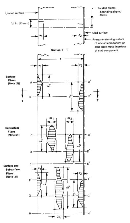
GENERAL NOTE: The flaw depth dimensions  $a_s$  and  $a_s$  are the allowable flaw standards for surface and subsurface flaws, respectively.
