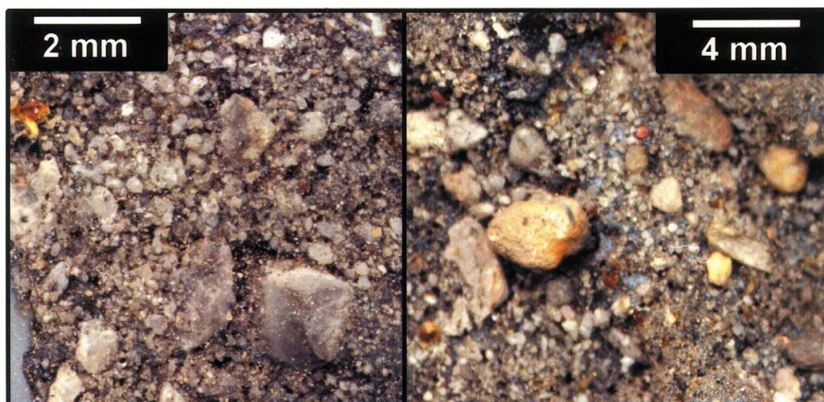
Fig. 11. Close-up photographs of experimental peperite textures, showing the intimate mixing of sand grains (from 65 to 70% by volume) within the thermite magma analog. Little or no thermal alteration is visible on any of the sand grains, evidence that quenching was rapid.
