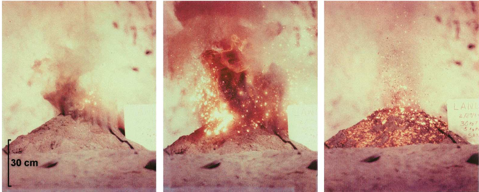
Fig. 6. A series of three photographs depicting the eruption produced by a Type 3 experimental design. The volcano edifice was constructed of sand and is about 0.5 m in diameter and 0.2 m high. Note the cm-size incandescent melt fragments following ballistic trajectories, the black finer grained melt quenched and carried up from the vent in convecting plumes while some moves downslope in a density current, and a small lava flow rivulet running downslope on the right.
