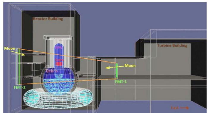
**Muon imaging setup for Fukushima Daiichi Unit 2. FMT-2 is installed inside a concrete radiation shield in front of the reactor building. Typical muon scattering angles are a few degrees.**
