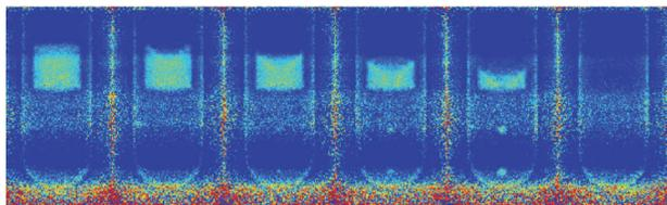
Results of the GEANT4 simulations for Unit 2. (From left to right): The simulations were run with intact core (left), 10%-, 30%-, 50%-, 70%-melted core and no core (right). Two spherical debris of 10-cm (under 10%-melted core), 20-cm, 30-cm and 40-cm (under 70%-melted core) radii were placed in the lower region of the reactor pressure vessel.
