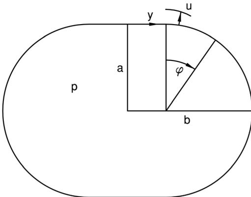
FIG. 7. The top-right quadrant of the thin shell runs clockwise from  $y = 0$  to  $y = b - a$  along the straight part and then from  $\phi = 0$  to  $\phi = \pi/2$  along the curved part. Internal pressure  $p$  causes deflection  $u$ , taken to be positive outward.
