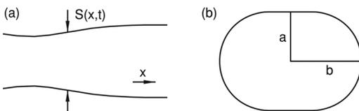
FIG. 2. (a) A tube extending in the  $x$  direction with a variable area  $S(x, t)$ . (b) A tube with racetrack-shaped oval cross section with semi-minor axis  $a$  and semi-major axis  $b$ .
