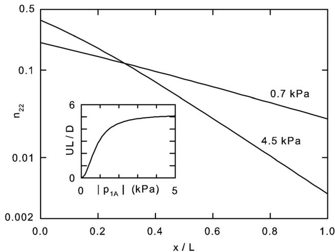
FIG. 9. Predicted  $x$  dependence of steady-state mole fraction  $n_{22}$  in our apparatus at the mid-tube pressure amplitude used for enrichment measurements shown in Fig. 6 (0.7 kPa) and at a higher amplitude that should be accessible with better tubing and drivers (4.5 kPa;  $|p_{1A}|/p_m = 0.05$ ). The average of each curve is  $n_{\text{fill}} = 0.092$ . Inset: The dependence of  $UL/D$  on pressure amplitude in our apparatus.
