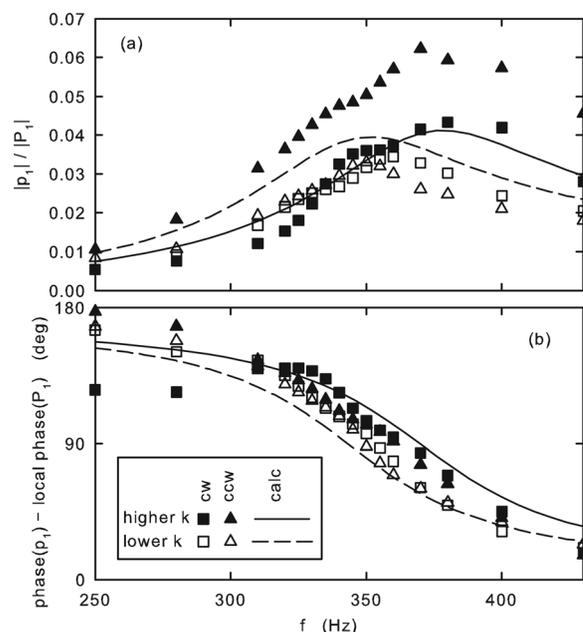
FIG. 3. (a) Relative magnitude and (b) relative phase of neon pressure  $p_1$  and water pressure  $P_1$  at the two locations 17.75 turns from the nearest end of the enrichment tube as functions of frequency  $f$ . Points represent measurements; curves represent Eq. (23). The measurements include two directions of wave propagation, which we call clockwise and counterclockwise.
