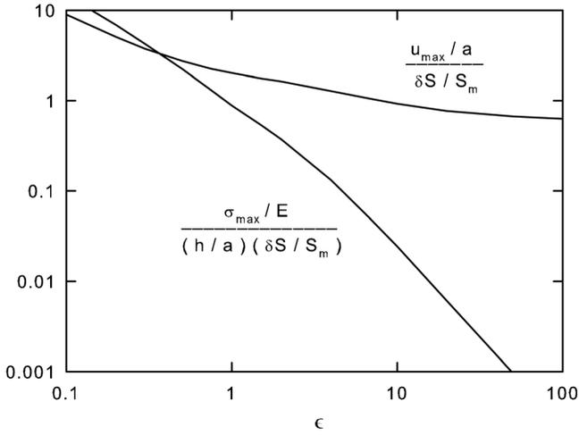
FIG. 8. The maximum displacement and maximum stress of the racetrack-shaped shell as functions of  $\varepsilon$ .
