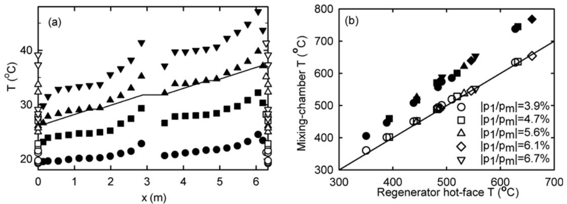
FIGURE 3. (a) Temperature  $T$  as a function of position  $x$  around the loop of Fig. 2(a), for four different heater powers. (b) Temperature of the steady flow entering (filled symbols) and leaving (open symbols) the mixing chamber of Fig. 2(b), as a function of the regenerator hot-face temperature.
