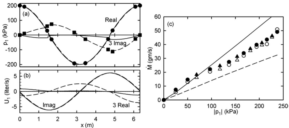
FIGURE 4. (a) Pressure and (b) volume flow in the one-wavelength loop. (c) Mass flow around loop.
