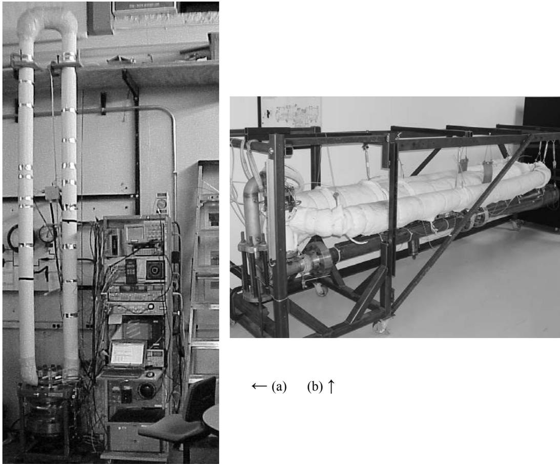
FIGURE 2. (a) Full-wavelength and (b) half-wavelength apparatus. White insulation covers both loops.
