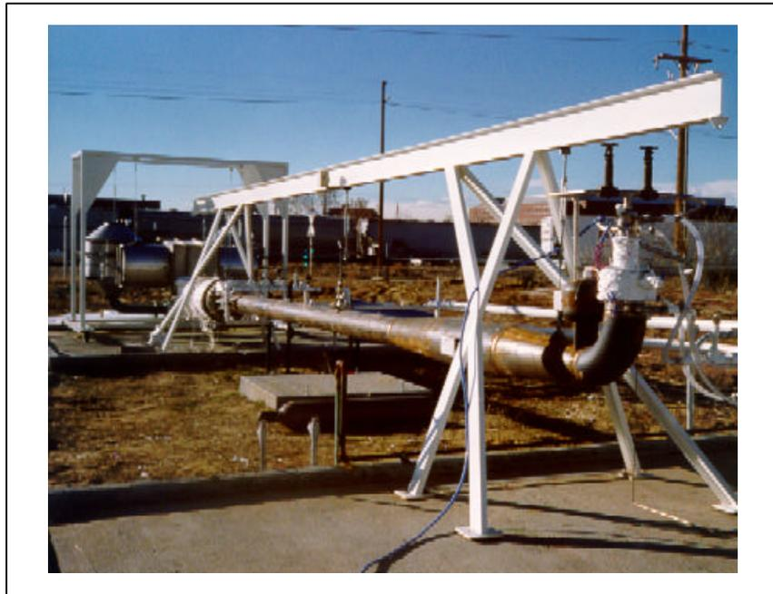
**Figure 1.** The 140 gpd TADOPTR Prototype
