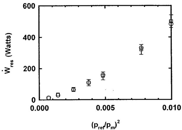
FIG. 11.  $\dot{W}_{res}$  measured (open squares) and calculated (open circles) vs  $(p_{ref}/p_m)^2$ . The DeltaE calculations use a relative surface roughness for the resonator of  $7 \times 10^{-5}$ . At low amplitudes, the error bars are smaller than the symbols.
