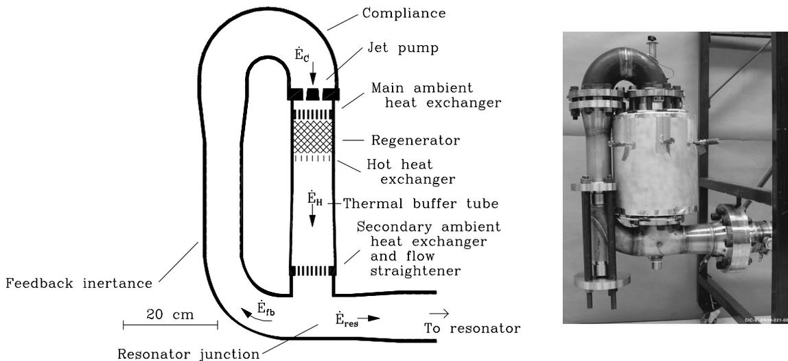
*Fig. 5. Thermoacoustic-Stirling hybrid engine, producing 1 kW of power at an efficiency of 30% without moving parts. The  $\dot{E}$ 's show the circulation and flow of acoustic power.*
