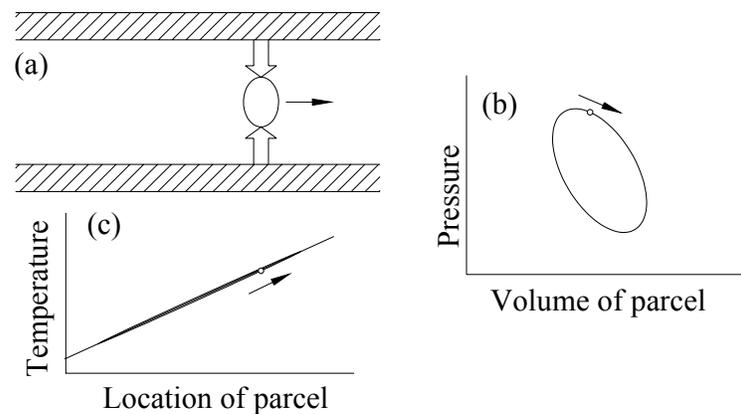
*Fig 4. The process in the regenerator of a traveling-wave engine. Note that temperature vs position and time is different from Fig. 2: Good thermal contact creates the clockwise pressure-volume ellipse via traveling-wave phasing here.*
