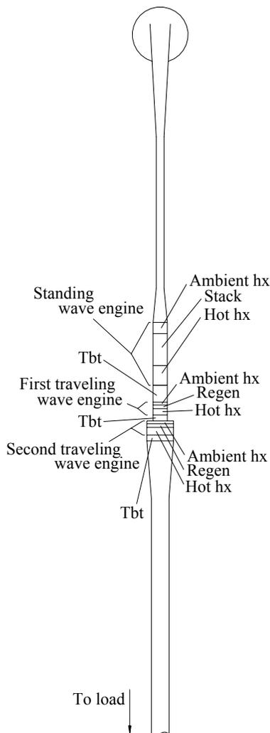
*Fig. 6. A cascade of one stack and two regenerators, with the necessary adjacent heat exchangers and intervening thermal buffer tubes, should provide high efficiency in a simple, reliable package. The portion of the resonator shown in the figure is approximately  $\lambda/2$  tall. "Tbt" is a thermal buffer tube, and "hx" is a heat exchanger.*
