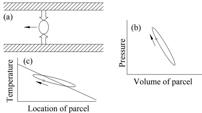
*Fig 2. The standing-wave engine process. (a) A parcel of gas oscillating horizontally in a channel. At this instant of time, it moves left (small arrow) and absorbs heat from the channel walls (large arrows). (c) The straight line shows temperature vs position in the channel walls, and the ellipse shows temperature vs position and time of the parcel. (b) Pressure and volume of the parcel trace out a clockwise ellipse as functions of time.*
