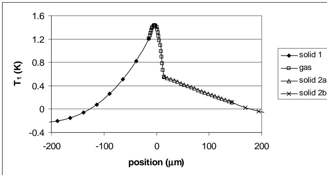
**FIGURE 3.** Temperature solution at 15 K using flow and pressures from the system model used in FIGURE 2.
