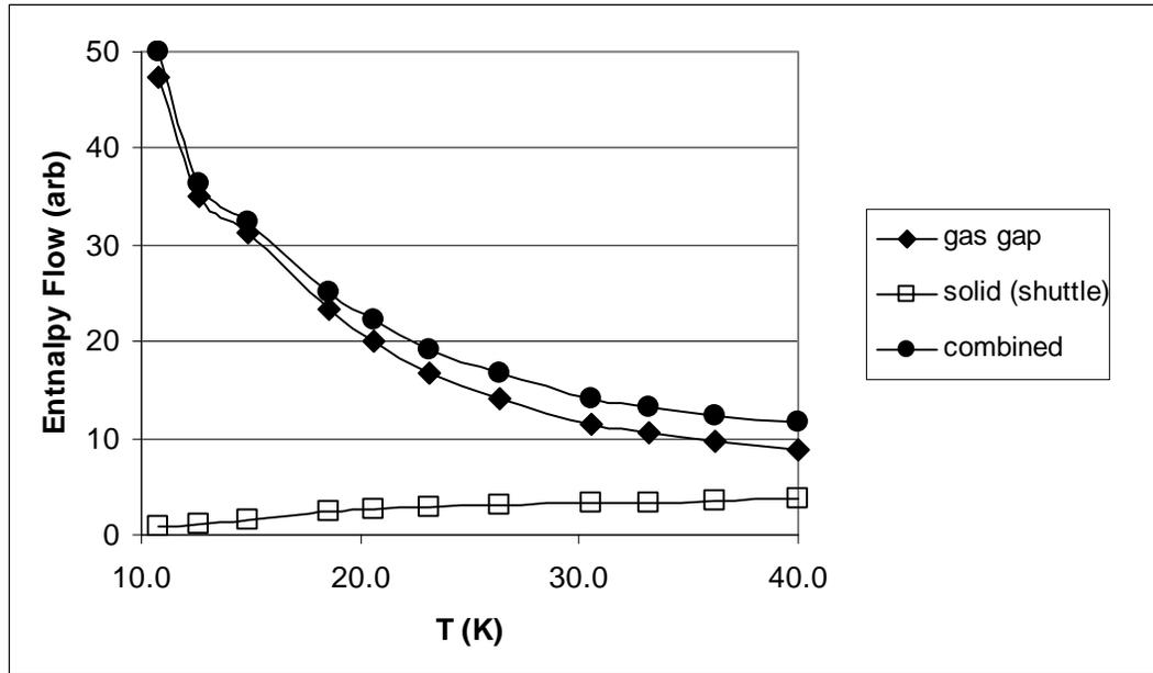
**FIGURE 4.** Enthalpy flow as a function of temperature showing a significant increase in gap loss as the temperature decreases.
