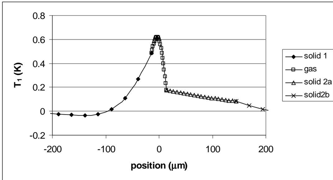
**FIGURE 2.** Temperature solution at 40 K at a particular time during a cycle. Wall velocity is zero, and the solid boundaries extend well beyond the scale on this plot.
