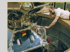
VELA satellite in Environmental Test Chamber. (1970)
