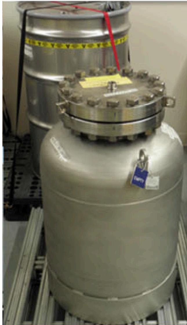
*The Flanged Tritium Waste Containers are pressure vessels specifically designed to contain waste metal that has been exposed to tritium. As the tritium ages and separates into helium and hydrogen, those gases can create pressure inside the container. This is expected and accounted for in the design.*
