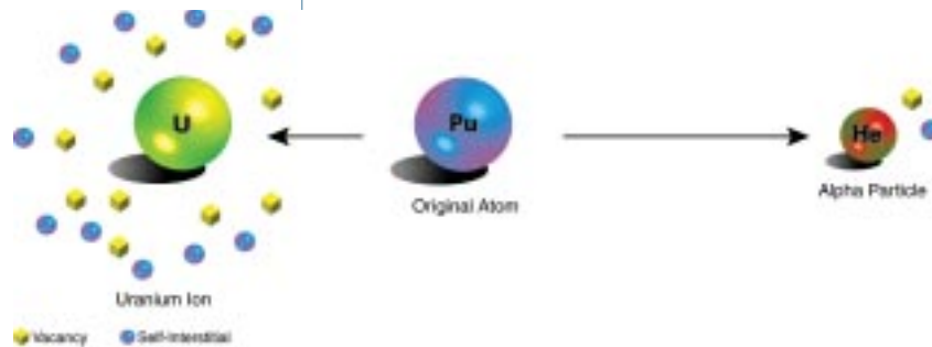
This schematic illustrates the radioactive decay process of a plutonium-239 atom. The alpha particle releases and the uranium-235 atom recoils.
