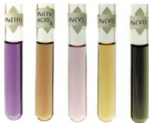
Figure 2. The color of plutonium oxidation states. Each oxidation state, ranging from Pu(III) to Pu(VII), has a characteristic color in solution. Plutonium will often change oxidation states in solution, making its interaction with the natural environment inordinately complex.
