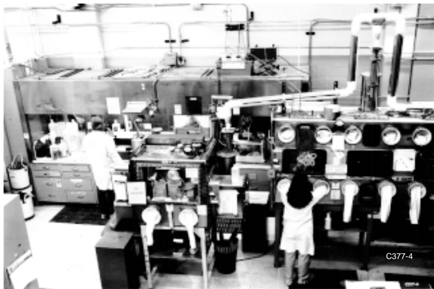
Figure 2. The Wing 9 fabrication line produces uranium targets that will be used for production of ^{99}\text{Mo} .
