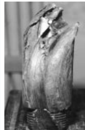
Figure 2. A damaged americium-beryllium neutron source recovered from a private company by Los Alamos.
