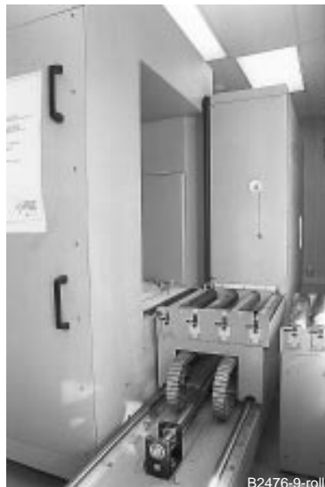
Figure 3: An imaging passive/active neutron counter in the Pajarito Scientific Corp. trailer.
