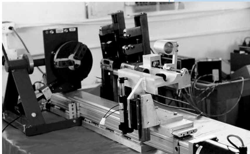
Figure 5: The remote decladder used in the Neutron Source Recovery Project reduces radiation exposures to personnel working on the disposal of unwanted radioactive neutron sources.
