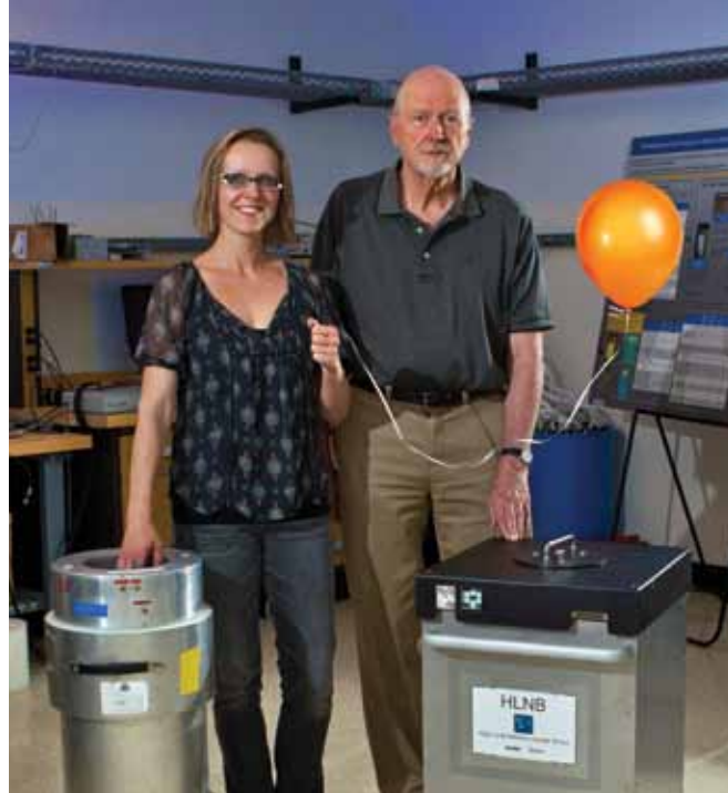
Daniela Henzlova and Howard Menlove celebrate their neutron detectors, new and old, with a helium-4 balloon. The helium-3-based high-level neutron coincidence counter (cylindrical, left), invented by Menlove in 1983, may soon be replaced in nuclear safeguards applications by their new boron-10-based coincidence counter (right).
