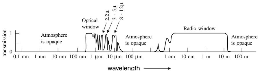
Note the “infrared windows” at  $2.2\mu, 3 - 5\mu, 8 - 12\mu$ , as well as the large optical and radio windows. UV and X-ray astronomy can only be done from space.
