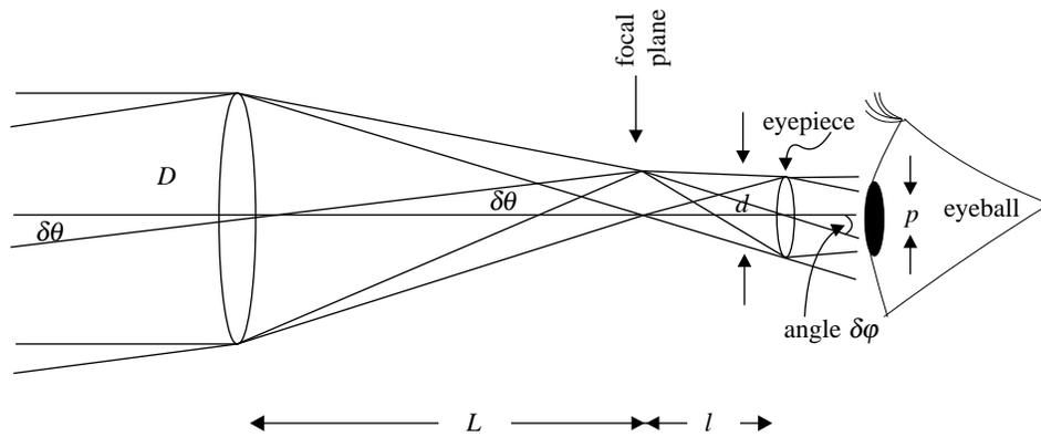
$D$  is the aperture;  $L$  is the focal length of the objective lens;  $d$  is the exit pupil;  $l$  is the eyepiece focal length
