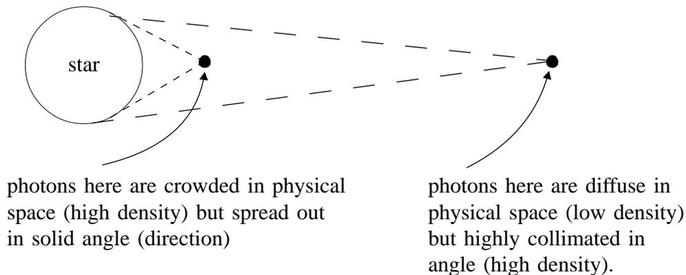
So, dilution of photon density is always accompanied by increased collimation in a precise quantitative relationship!
