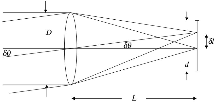
This is the basic “prime focus” astronomical telescope. The detector (CCD array) goes at the focus. The “image scale” is the ratio of physical distance at the focus to angular distance in the sky, and it depends *only on the focal length* (see figure),
