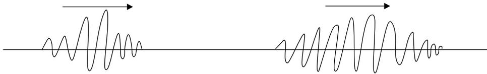
The more monochromatic (small  $\Delta E$  or  $\Delta\nu$ ) the photon, the longer the wave packet. This is why it is easy to do interference demonstrations with laser light (very monochromatic) but quite difficult with white light (large  $\Delta\nu$ ). The relation between length of wave packet and frequency (or energy, or momentum) localization is of course the Heisenberg uncertainty principle.
