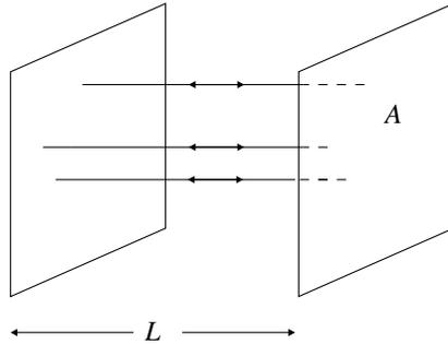
Each photon contributes  $\Delta u = E/(AL)$  to the energy density (since the volume is  $AL$ ). Each photon gives a momentum transfer  $2p$  each time it bounces off the mirror ( $+p$  goes to  $-p$ , so the difference is  $2p$ ). These bounces occur (on a given mirror) every  $2L/c$  time, so the photon's contribution to the pressure is
