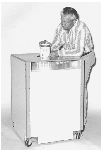
Fig. 6.1. Photo of the Plutonium Scrap Multiplicity Counter, used for accurate assays of plutonium metal, oxide, mixed oxide, or scrap.
