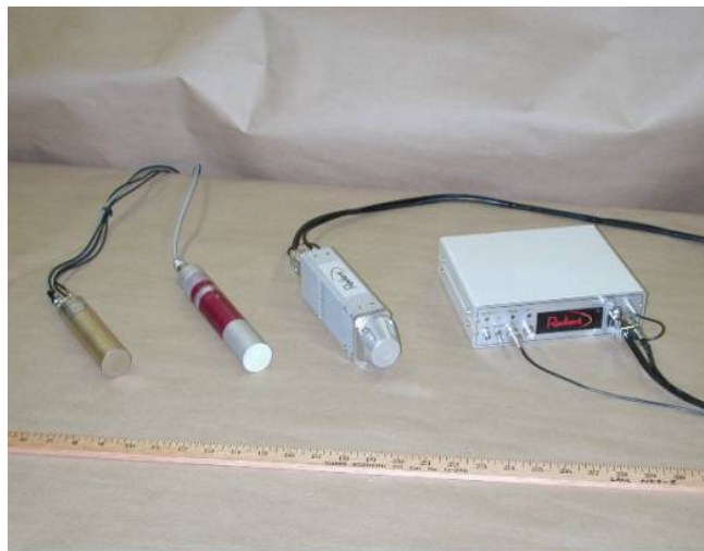
Fig. 14. The CPG CdZnTe, compact NaI, and CdTe detectors (Table 7) pictured at the left, center, and right, respectively. The rectangular module at the right is the power supply for the Peltier cooler within CdTe detector.
