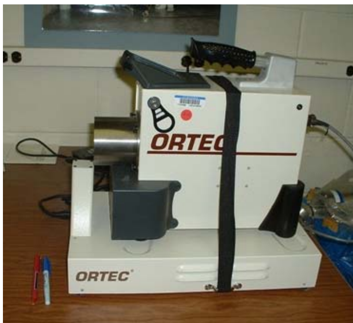
Fig. 10. The portable electrically-cooled Ge detector with tungsten collimator is shown mounted on a docking station (rectangular base) used for charging and cool down. The weight without the docking station is 12 kg.
