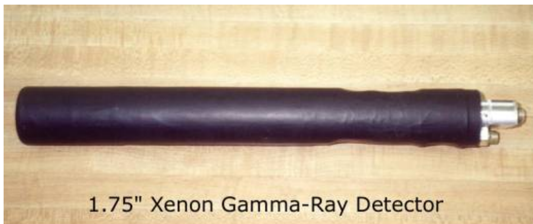
Fig. 18. Commercial prototype HPXe detector. The diameter and active length are 4.5 and 10 cm.
