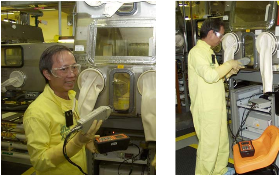
Fig. 15. A Peltier-cooled CdTe detector and DSP MCA in use for isotopics measurements Pu in a glove box.
