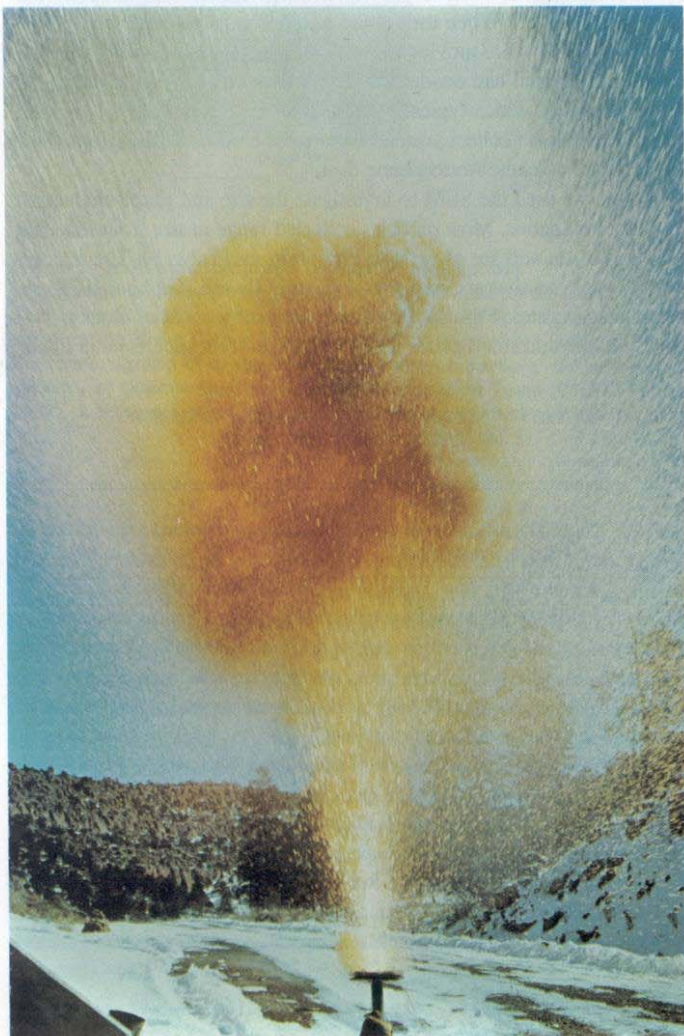
Figure 1. Photographs of top-venting experiment exhibiting explosive behavior. Left: Frame obtained \sim 1 s after burst time. Right: Frame obtained \sim 1.5 s after burst time.
