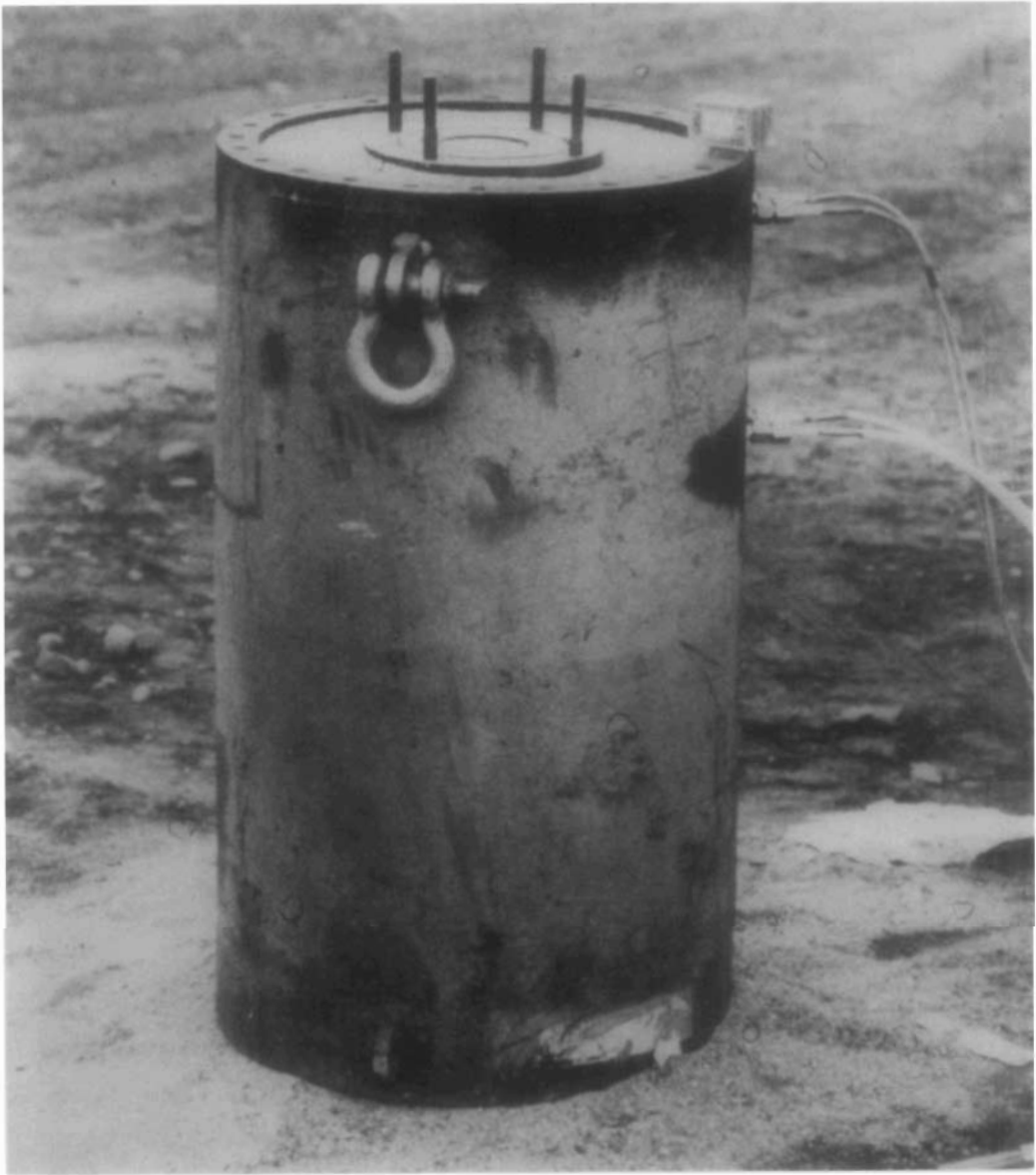
FIG. 5. Steel vessel used in the thermite-water experiments. Note the connectors for P - T readout. A Kodak film box is shown for scale.
