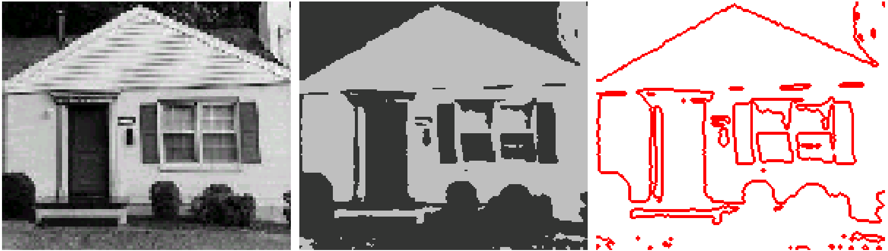
Original grayscale image of a house (left); CVT-based segmentation into two segments with subsequent averaging (middle); the corresponding edges (right)
