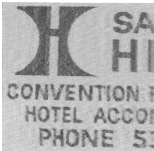
Figure 5. In a typical example of the power of digital image processing, linear MAP restoration of a photograph a) that is subjected to linear-motion blur, produces an eminently readable result b).
