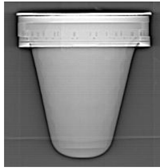
(b) A breast phantom with many inclusions
