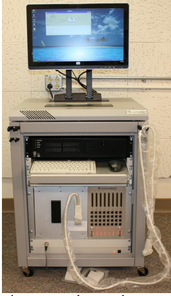
Figure 1: Our custom built, real-time synthetic-aperture ultrasound system (InnerVision DAS009) with a Prosonic HL5-10/40EPN transducer. The machine has a maximum frame rate of 25 Hz, and is capable of acquiring synthetic-aperture ultrasound data and forming ultrasound images in real time.
