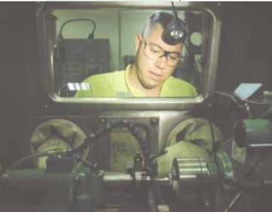
*Chris Trujillo of the Nuclear Materials Science Group (NMT-16) machines a Kolsky test specimen. A non-water-based coolant is used to flood the specimen during machining. Flooding ensures that the sample is not overheated during the machining process, avoiding the introduction of nonaging-related artifacts into the plutonium sample.*
