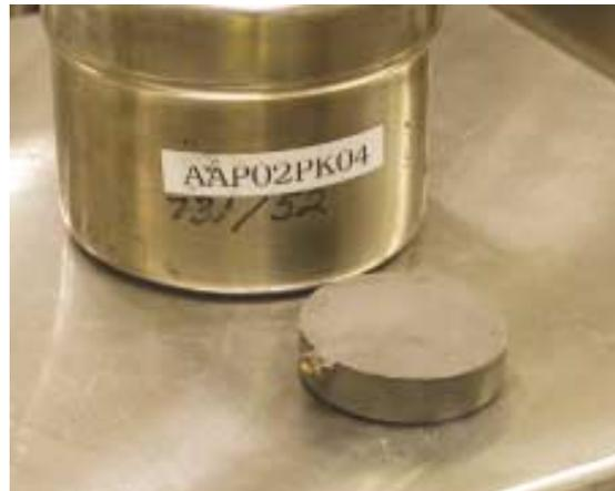
*The casting yielded nine enriched plutonium "cookies," one of which is shown here. The thickness of this miniature ingot duplicates the thickness of the Rocky Flats ingots, giving researchers a good simulant for the next stage of processing: rolling the ingot into a sheet.*
