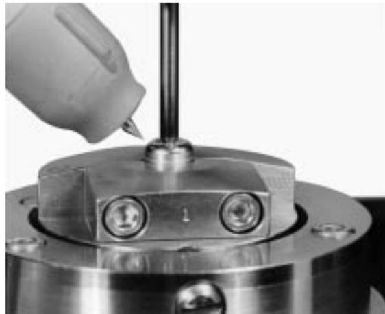
**Figure 2.** The LWRHU assembly consists of the fueled capsule, three layers of pyrolytic graphite thermal insulation, and the outer, impact-resistant graphite fiber aeroshell. Three of these heat sources were recently used to keep electronics at normal operating temperature on the Mars Pathfinder rover, and 117 are on their way to Saturn on the Cassini spacecraft.
