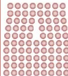
**Figure 3. Energy deposited in the metal lattice produces disordered regions including dislocations and vacancies. Such damage can alter the mechanical properties of a metal through a complicated set of competing processes. This figure shows dislocation in the lattice as a result of a damage cascade.**
