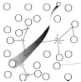
lision phase” process produces a large region in which the lattice has been disrupted, producing dislocations, interstitial atoms, vacancies, and other lattice defects.
