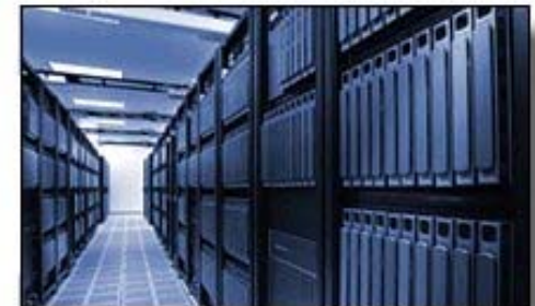
2,304 Intel® Xeon™ 2.4 GHz processors power this 5.69 TFlops supercomputer at Lawrence Livermore National Labs. It rates as the fifth fastest in the world.
