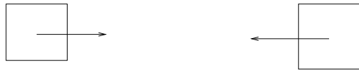
Figure 4: Dot product is negative between the two area vectors, so they face each other
