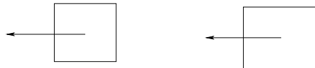
Figure 5: Dot product is positive, so one of the faces is in the wrong direction.
